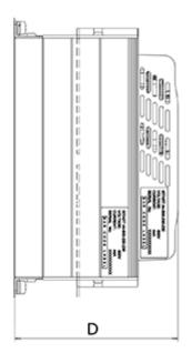
Control voltage (terminal A1, A2) = 230AC D = 275 Digital control voltage (terminal 1-5) = 24DC H = 645 Kg = 37 W = 365
